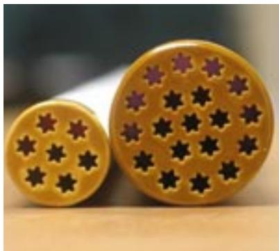
With a constant crossflow velocity, it is beneficial to design the filter channels with maximum circumference (or perimeter), giving rise to a greater membrane area. At the same time, it is important that the filter channels are designed with a minimum cross-sectional area in order to reduce the retentate flow required to maintain this constant velocity.
