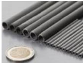
The tubular membranes are laser welded into a 316L housing for membrane areas of 0.5 – 10 m<sup>2</sup>. The tubes can be used as such, as well as coated with a proprietary stainless steel or ceramic layer. Pore size range in this way is from > 10 micron down to 20 nm allowing a broad range of filtration applications including Food & Beverage, Dairy, Membrane Bioreactors, Clarification Processes, Pharmacy, Water Treatment and Gas Filtration (PM 2.5).
