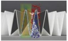
the entire process chain from the fiber laydown process to the final filter material can be established. This enables the users to optimize and control the product quality in terms of flow resistivity and filter performance, leading to a more efficient and reliable manufacturing. In addition, Fraunhofer ITWM develops FeelMath, a structural mechanics solver specialized in compound and porous materials and PoreChem, a simulation tool for reactive flows in porous structures.
